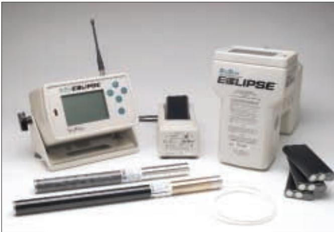
An HDD locator system (from the left): the remote display, a battery charger with a rechargable Ni-Cad battery, Eclipse receiver, followed by a stack of batteries. In the foreground are two transmitters, a battery powered one (closest to the system) and then a cable transmitter (longer with a wire attached).
