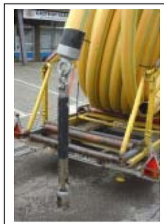
Figure 4. TensiTrak load monitor attached to the reel ready to start logging data.
