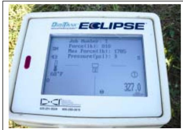
Figure 3. Typical Eclipse receiver display while in TensiTrak mode.
