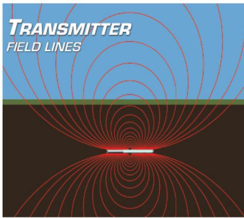
Di-pole electro-magnetic field emitted from an HD transmitter.
