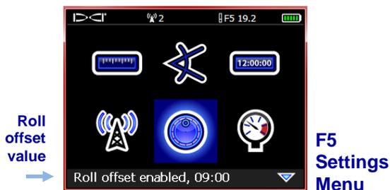
Tap or drag on the roll indicator in the app to select the roll offset value, then tap **Start**. Tap **Start** again on the 10-2-7 screen and roll the transmitter within the allotted time to the flashing blue band at the 10:00 position, then wait as instructed.
