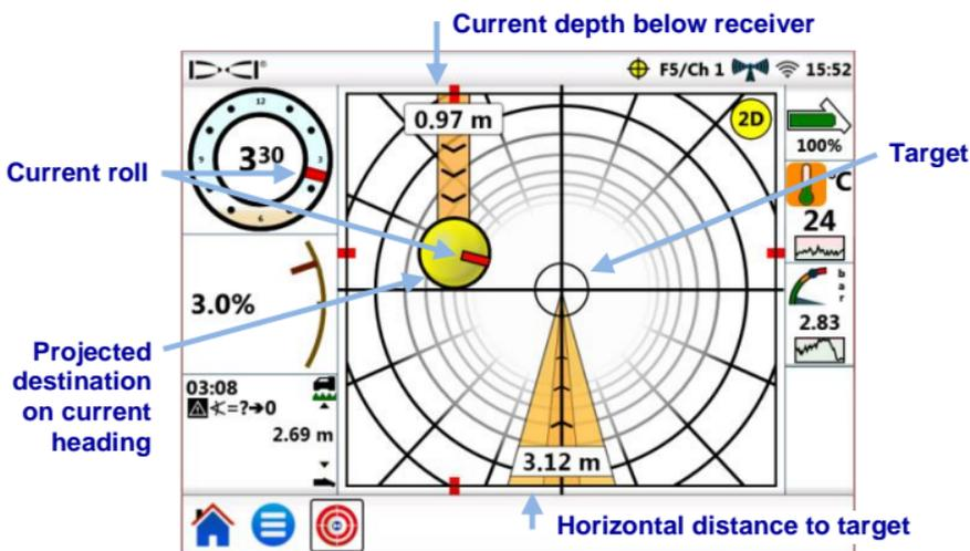
Steer the yellow steering indicator ball (the projected destination) onto the target. In this case, the drill head is currently estimated at 0.97 m below the plane of the receiver and must travel 3.12 m to reach the target point below the receiver.
