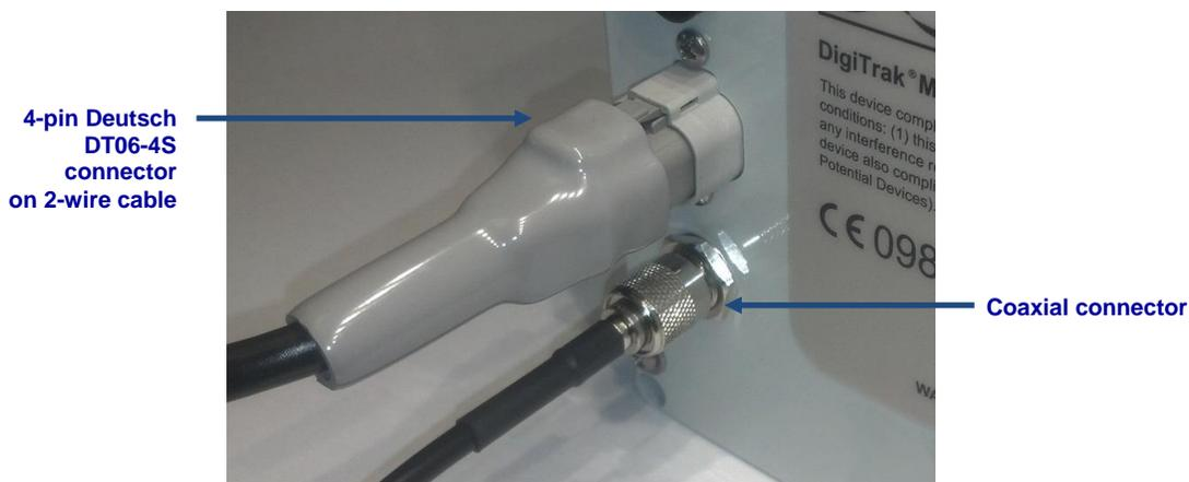
**Power and Antenna Connections on Back of DigiTrak MFDp**
